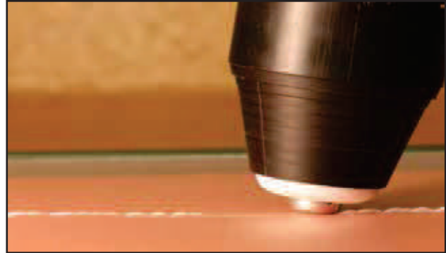
An eraser rests on the plastic and is moved back-and-forth to flatten raised-lines
